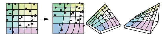
It can be useful to sample from the *bilinear interpolation function*, which we define as taking four values v[4] that define a function over  $[0, 1]^2$  by
