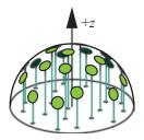
A common way to generate diffuse rays in rendering methods for matte surfaces is to sample uniformly from a disk (as in Section 16.5.1) and then project the sample point up to the hemisphere. Doing so produces samples with a *cosine-weighted* distribution, where the density is high at the apex of the hemisphere and falls off toward the base. Generated samples will need to be transformed into the local tangent space of the surface being rendered.
