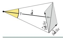
**Figure 21-2.** When disregarding the differentials of the ray origin, the spread angle  $\gamma$  can be computed using the normalized ray direction  $\hat{d}$  and its differentials.
