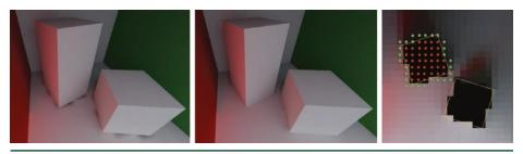
**Figure 23-9.** Dilation filter applied to a light-mapped Cornell box. Left: texels covered by geometries have invalid irradiance, due to paths hitting inner geometry, which is flagged as invalid. Middle: a dilation filter is applied for removing invalid texels. Right: top view of the scene showing the valid texels (green) and the invalid texels (red) for one of the objects.
