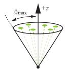
Given a cone with axis along the +z-axis and a spread angle  $\theta_{\max}$ , uniform directions in the cone can be sampled as follows:
