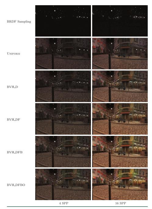
**Figure 18-9.** Visual results at 4 samples per pixel (SPP) (left) and 16 SPP (right), using the different sampling strategies defined in Section 18.4.3. All BVH-based methods use a BVH built with SAOH evaluated for 16 bins along all axes. The BVH techniques use MIS: half their samples sample the BRDF and half traverse the light acceleration structure.
