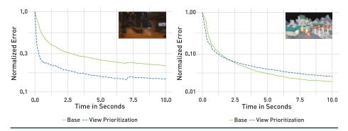
**Figure 23-18.** Plots illustrating the converge gain obtained by denoising the light map output on two scenes: Granary by Night (left) and Zen Peak (right). These plots show the relative error (L1) compared to a reference light map. This denoising step removes most of the high- and medium- frequency noise and allows us to quickly present a result similar to the converged output.
