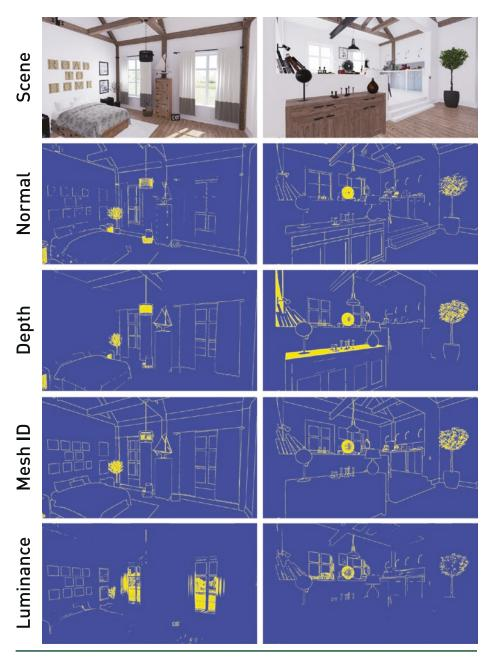
**Figure 22-5.** Segmentation results of 3 × 3 pixel convolutions for various types of screen-space data from two viewpoints in the Modern House scene: from top to bottom, final shaded scene, surface normals, depth, mesh identifiers, and luminance.
