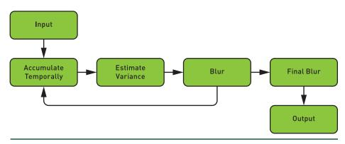
Figure 25-6. Shadow filtering, inspired by the work of Schied et al. [24].
