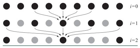
**Figure 24-5.** Three iterations of the one-dimensional stationary wavelet transform that forms the basis of the Á-Trous approach. Arrows show the nonzero elements of the previous result contributing to the current element, while gray dots indicate zero elements. (Illustration after Dammertz et al. [4].)
