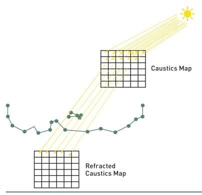
**Figure 14-10.** Ray tracing a refracted caustics map: send rays from the water surface positions stored in the caustics map along the refracted light directions, and store the resulting ray/scene intersections in a refracted caustics map.
