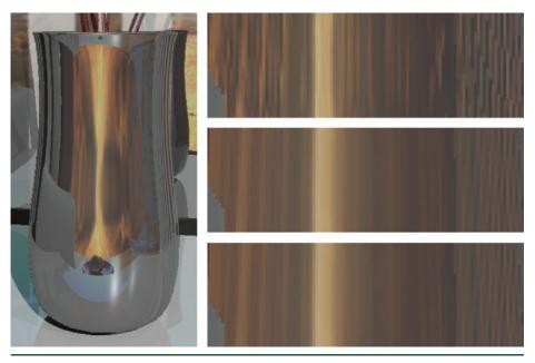
**Figure 21-3.** A vase with exaggerated reflections from an environment map (mostly brown area) using different methods. The closeups show, from top to bottom, use of mip level 0, ray cones, and ray differentials. Note that the two latter images are similar, which is expected since they filter the environment map. During animation, severe aliasing occurs in the image on the top right, while the other two are temporally stable.
