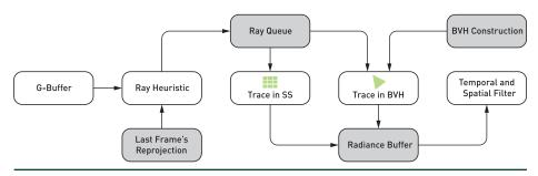
Figure 26-2. Overview of the ray creation scheme for both diffuse and specular BRDFs.
