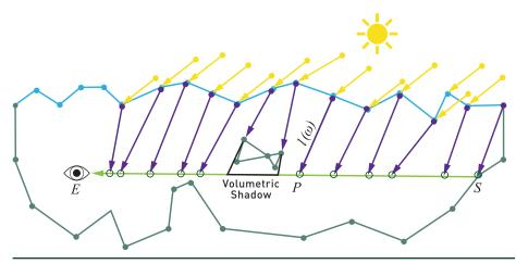
**Figure 14-4.** The eye *E* on the left looks to the right through the water. Light from above reaches various different locations along this ray, depending on the water's surface, and scatters light toward the eye.
