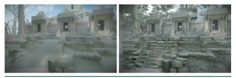
**Figure 23-2.** Light map applied to a scene in Star Wars Battlefront II. Left: light map applied to proxy meshes, against which GI is traced. Right: light map applied to final in-game meshes by projecting proxy UV coordinates and using normal mapping. (Courtesy of DICE, © 2018 Electronic Arts Inc.)
