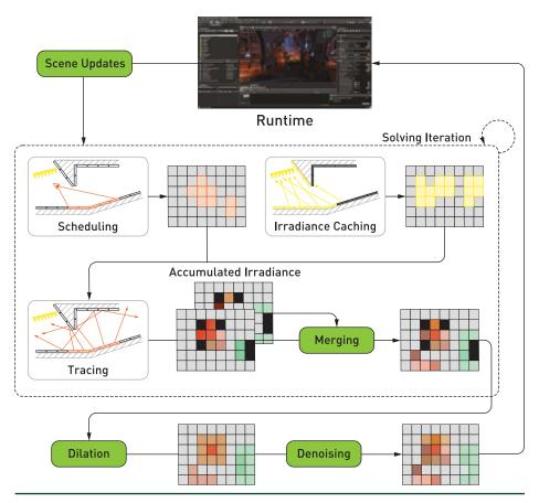
**Figure 23-5.** Overview of the GI solver pipeline. Light maps and irradiance volumes are updated iteratively. The camera viewpoint is used to prioritize texels that need to be scheduled for the tracing steps. Using an irradiance cache, the tracing step refines the GI data. The traced results are merged with those of previous frames, before being post-processed (dilated and denoised) and sent back to the runtime.
