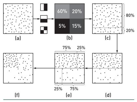
**Figure 24-3.** Warping a set of sampling positions by an iteration of the wavelet transformation. (a) The initial sampling positions are (c-d) first warped horizontally and (e-f) then vertically using (b) the ratios of the scaling coefficients in the active quad. (Illustration after Clarberg et al. [1].)
