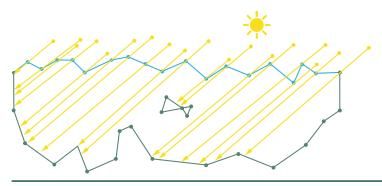
Figure 14-1. Undisturbed light rays hitting the underwater scene.
