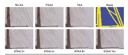
**Figure 22-7.** Zoomed images from the Modern House scene highlighting a challenging area featuring thin rope geometry, comparing boat rope details rendered with 1 SPP rasterization, FXAA, UE4's stock TAA, a visualization of our segmentation mask, ATAA 2×, 4×, and 8×, and an SSAA 16× reference.
