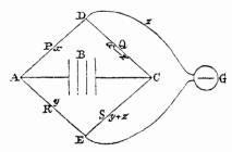
four remaining conductors are represented by P, Q, R, S, and the currents in them by x, x-z, y, and y+z, the current through G will be z. Let the potentials at the four points be A, C, D, E. Then the conditions of steady currents may be found from the equations
