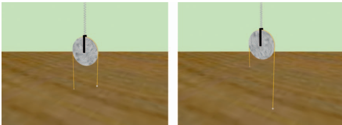
Color Plate 3.14 A mass pulley spring system shown at two different times. The spring expands and compresses and the pulley disk rotates during the simulation. The system stops when a mass reaches the center line of the pulley or the ground.
