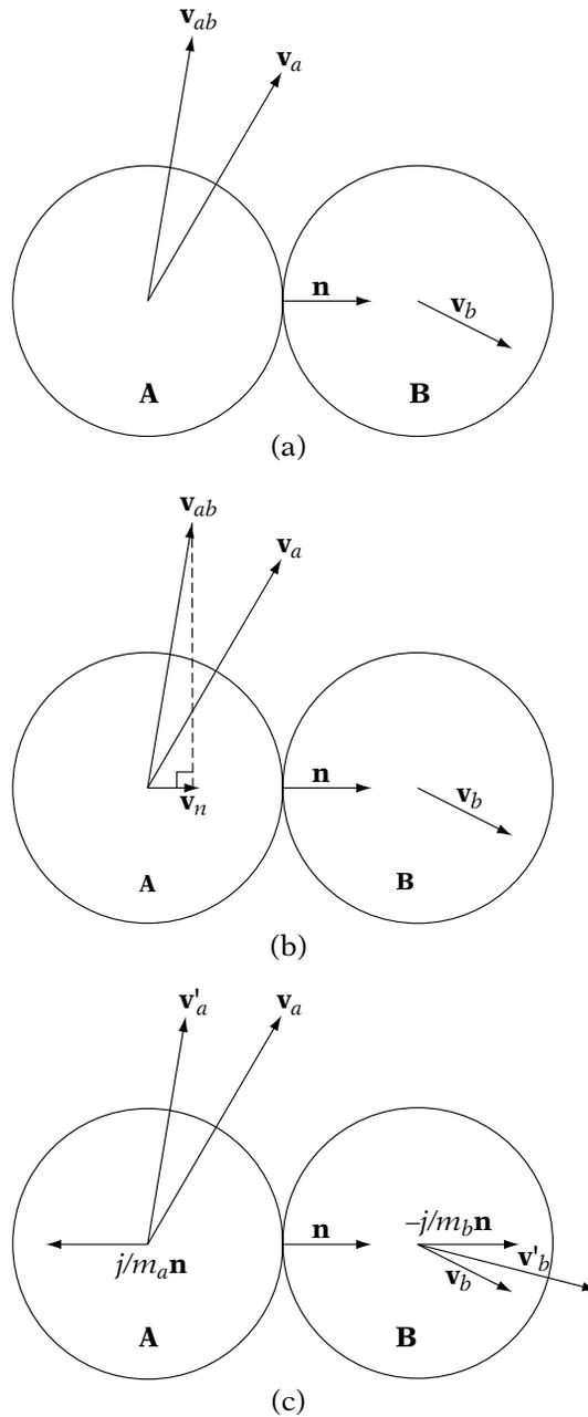
**FIGURE 13.16** (a) Computing collision response. Calculating relative velocity. (b) Collision response. Computing relative velocity along normal. (c) Collision response. Adding impulses to create outgoing velocities.
