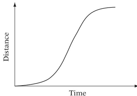
**FIGURE 10.28** Example of distance–time graph: Ease-in/ease-out function.
