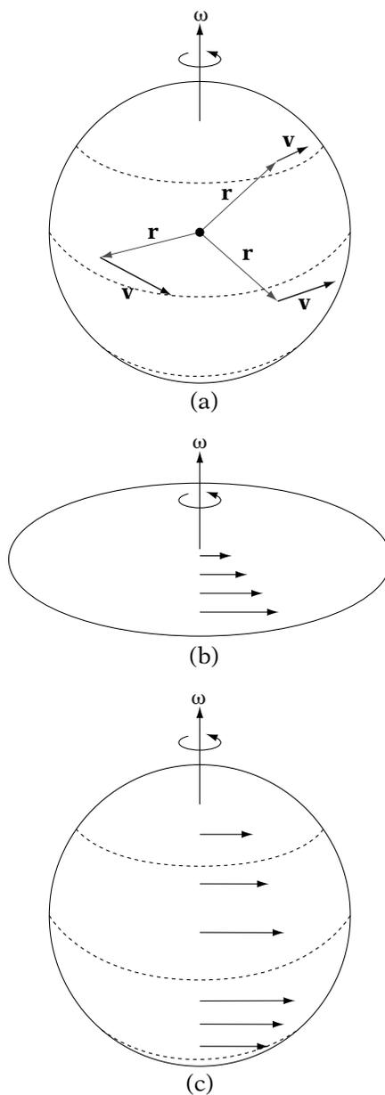
**FIGURE 13.10** (a) Linear velocity of points on the surface of a rotating sphere. Velocity is orthogonal to both angular velocity vector and displacement vector from the center of rotation. (b) Comparison of speed of points on surface of rotating disk. Points further from the center of rotation have larger linear velocity. (c) Comparison of speed of points on surface of rotating sphere. Points closer to the equator of the sphere have larger linear velocity.
