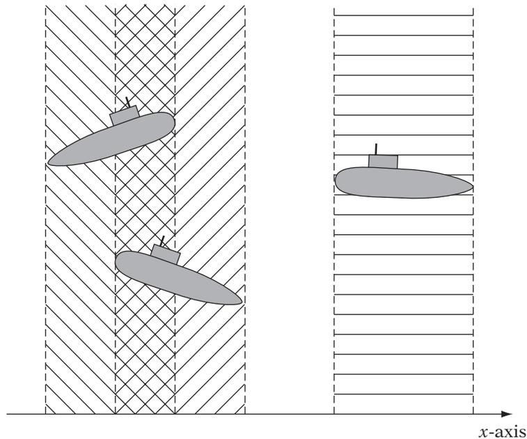
**FIGURE 12.29** Dividing collision space by sweep and prune.
