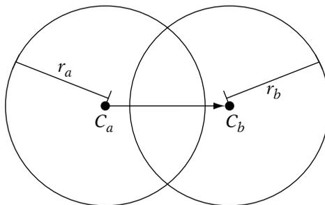
**FIGURE 13.15** Determining penetration distance and collision normal.
