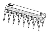
This is a 16-pin chip. If you hold the chip so the little indentation is at the left (as shown), the pins are numbered 1 through 16 beginning at the lower left and circling around the right side to end with pin 16 at the upper left. The pins on each side are exactly 1/10 inch apart.
