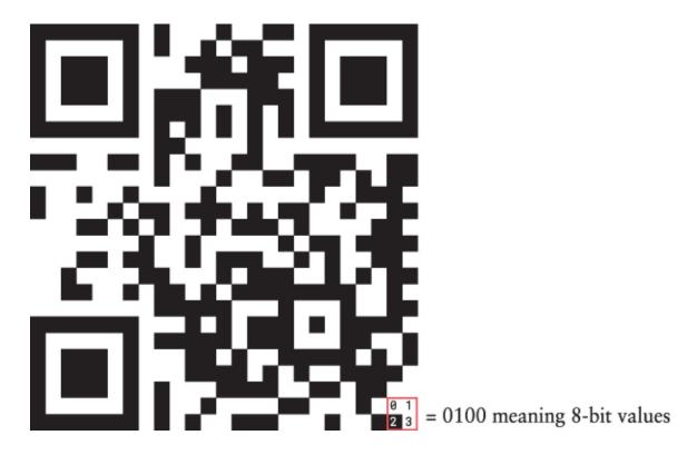
These four bits are known as the *data type* indicator, and they indicate what kind of data is encoded in the QR code. Here are a few of the possible values:
