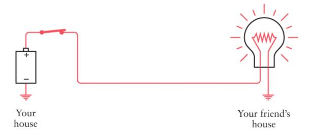
The electrons come out of the earth at your friend's house, go through the lightbulb and wire, pass through the switch at your house, and then go into the positive terminal of the battery. Electrons from the negative terminal of the battery go into the earth.
