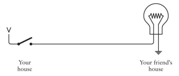
The V stands for *voltage*, but in a sense, it could also stand for *vacuum*. You can think of the V as an electron vacuum cleaner and think of the ground as an ocean of electrons. The electron vacuum pulls the electrons from the earth through the circuit, doing work along the way (such as lighting a lightbulb).
