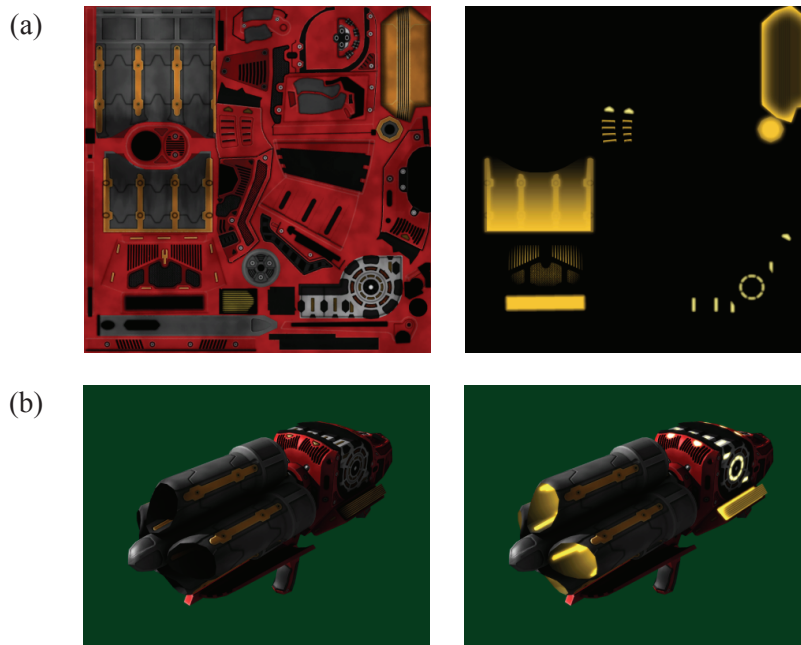
Figure 7.12. (a) The left image is an ordinary texture map, and the right image is an emission map. (b) The model on the left has only the ordinary texture map applied to it. The model on the right includes the emission map. Unlike the ordinary texture map, the emission map is unaffected by the direction of the surface normal, and it determines which parts of the surface appear to give off a glow. (Image from the game The 31st , courtesy of Terathon Software LLC.)
