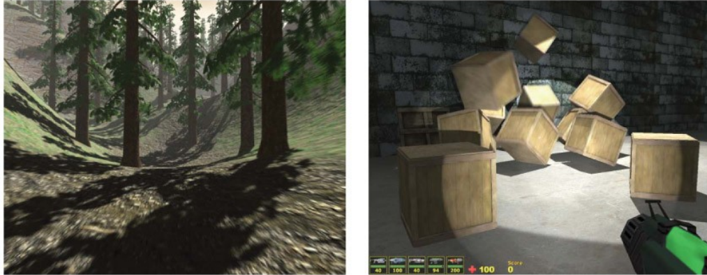
Figure 17.1: (See also Color Plates.) In the left image, motion blur resulting only from camera movement is shown. Notice how the ground and trees closer to the camera are blurred much more than distant objects. In the right image, motion blur resulting from rigid objects moving in the scene is shown. Both translational and rotational motion are visible in this still image. (Images courtesy of Terathon Software LLC.)
