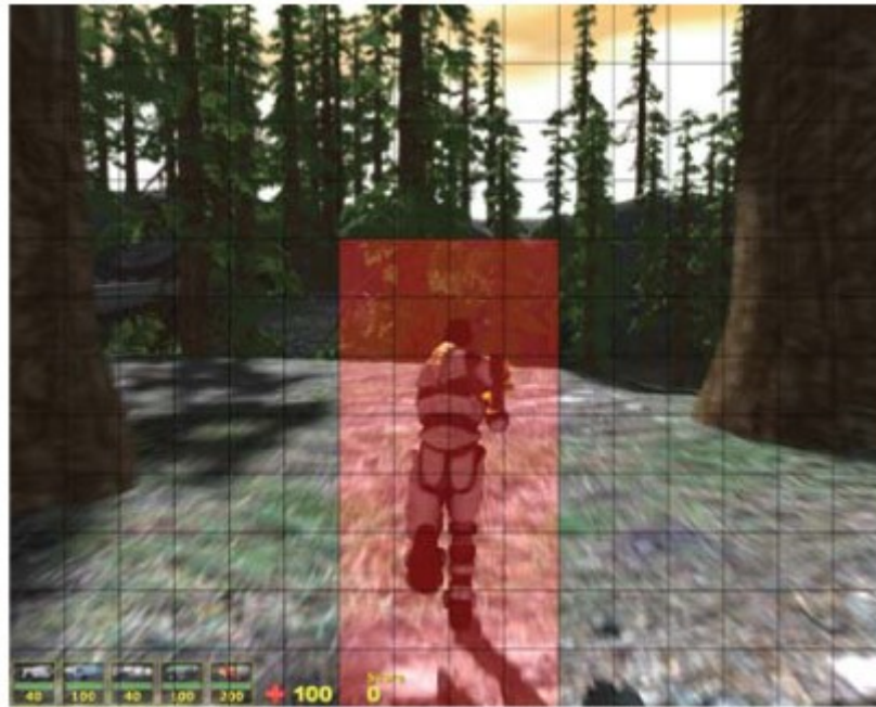
Figure 17.4: (See also Color Plates.) In this image, the viewport is partitioned into a grid of 16 \times 12 cells. The depth and gradient information is only used in the highlighted cells surrounding the character since that is where foreground objects are likely to be moving slowly relative to the background. (Image courtesy of Terathon Software LLC.)
