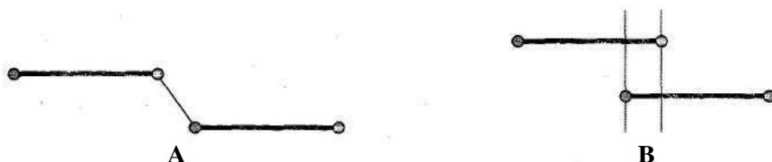
FIGURE 2.3.3 Parallel line segments. A) Unique nearest point pair. B) Locus of nearest point pairs.
