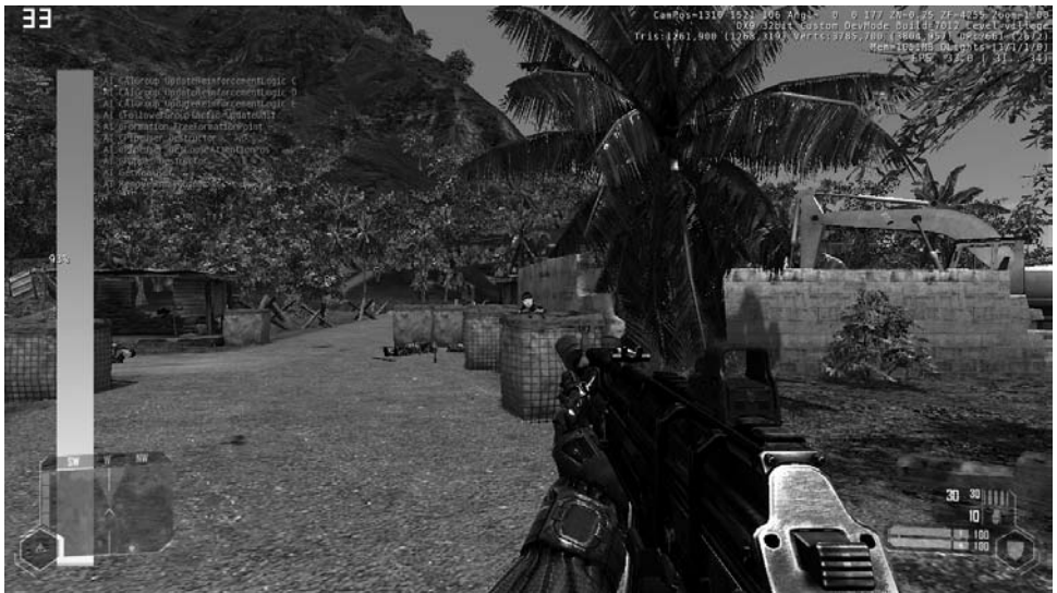
Figure 4.8.2 Code coverage within CryENGINE , when 93 percent of markers for the level have already been hit and the remainder are displayed as hints to the tester.
