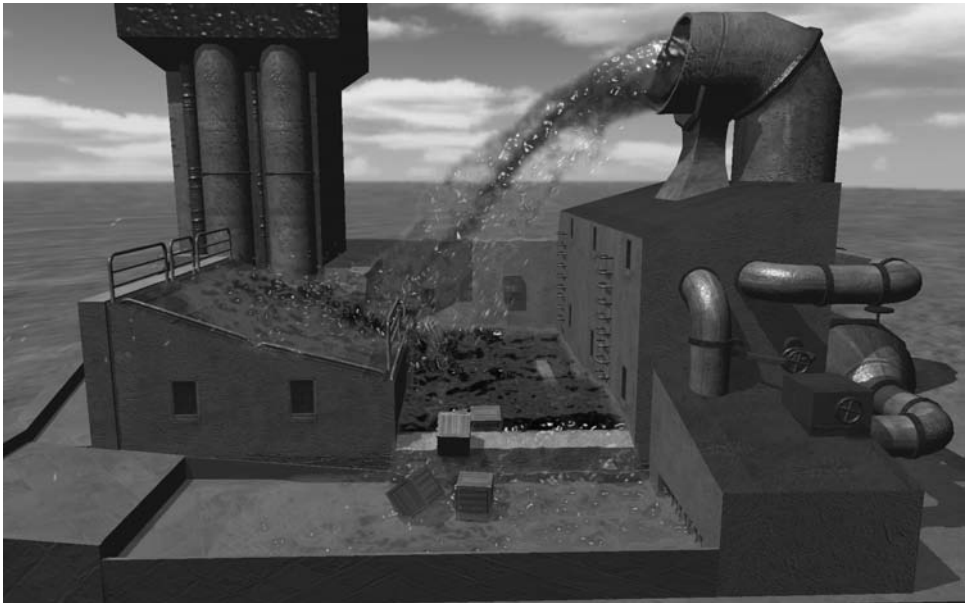
Figure 7.3.1 Real-time GPU-accelerated Smoothed Particle Hydrodynamics (SPH) water simulation in PhysX. There are more than 60,000 particles in the simulation. The rendering is performed using a screen-space splatting technique.
