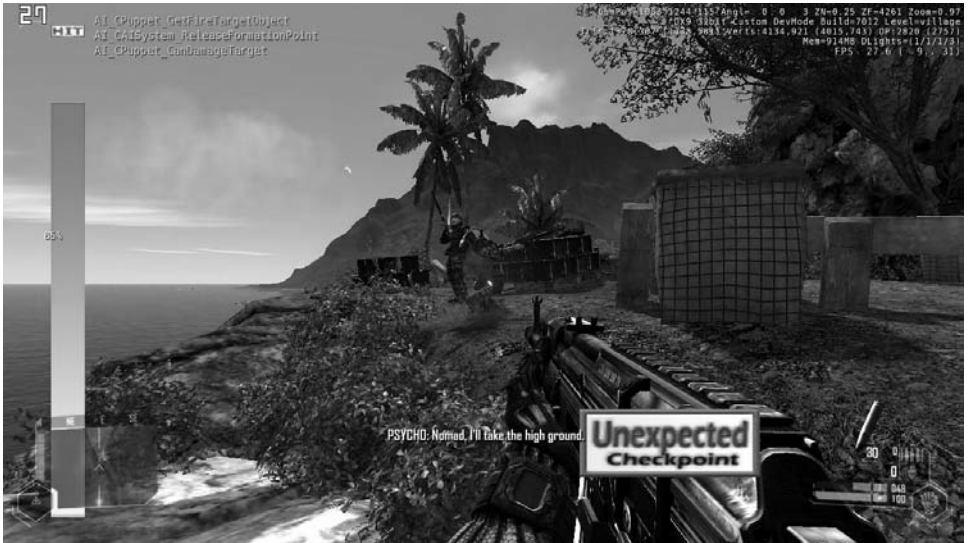
Figure 4.8.1 Code coverage GUI implementation within CryENGINE , including progress bar, hit indicators, and a list of markers hit within the last few seconds.
