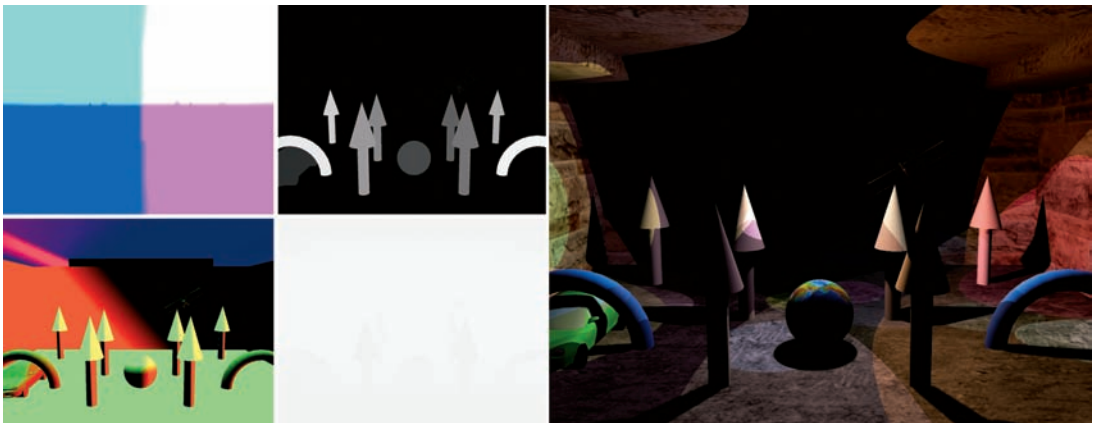
Color Plate 3: Output of rendering stages and final image from the deferred rendering technique described in Gem 1.3. Position and material ID (top left), normal and depth G-buffers (bottom left), and a resultant image (right).
