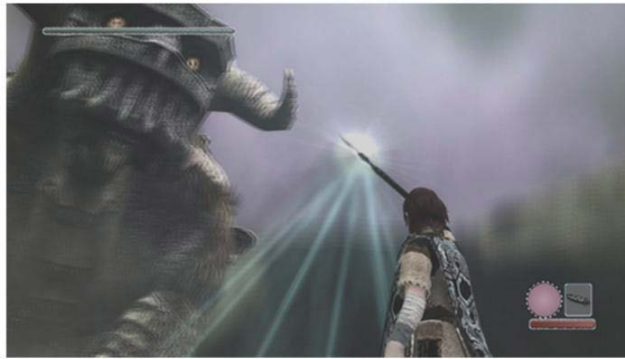
Figure 9.6. The adaptive dynamic algorithm remains focused on the character in most cases, adjusting the parallax separation based on the ratio of pixels in each category. This screenshot has mostly pixels in the far category. Consequently, the algorithm increases the parallax separation to increase the sense of depth. Notice that the UI elements are at the focal distance as well, but look good to the player because everything else is at or behind them in depth. (Image courtesy of Sony Computer Entertainment, Inc.)
