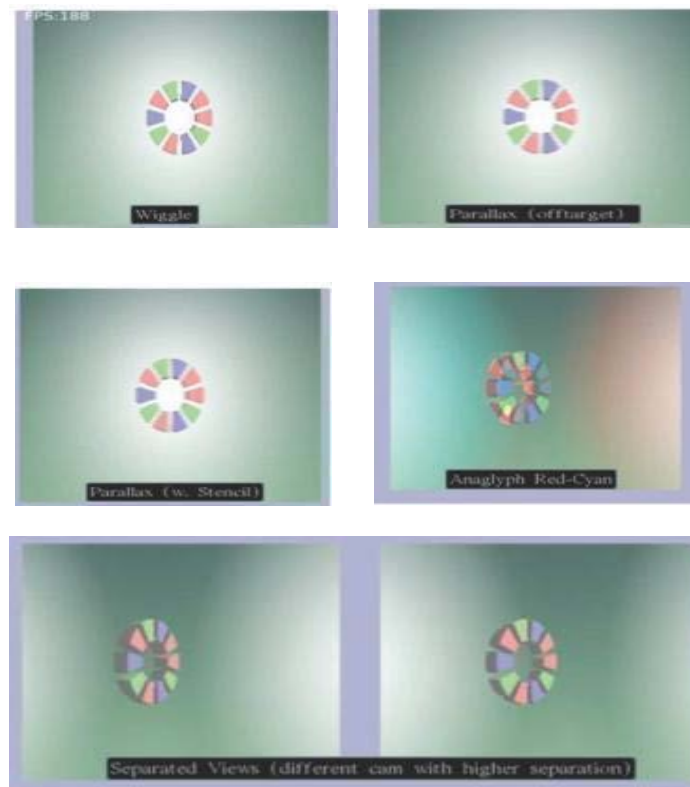
Figure 12.4. The same scene rendered to different viewports with different multiview configurations: anaglyph using color-mode (bottom-left), parallax using both off-target and on-target (stenciling), on-target-wiggle, and on-target-separated.
