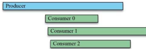
Figure 31.3. Sample timeline for producer-consumer model from Figure 31.2.
