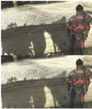
Figure 7.8. Leveraging the spatiotemporal coherency of shadows (bottom) enables a soft, filtered, look free of undersampling artifacts, without raising the shadow map resolution of the original scene (top).
