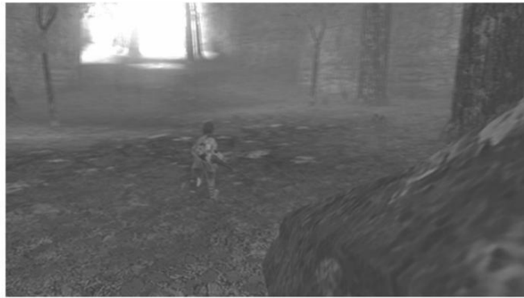
Figure 9.9. In this case, a large rock is very close to the camera. Setting the focal distance farther away than the rock would increase the pixels that would fall in the near category, causing the focal distance to shorten significantly. This self-correcting feedback is what allows for extremely dynamic environments to be handled comfortably. It effectively stops window violations in most cases, and it prevents uncomfortable protrusions toward the viewer. ( Image courtesy of Sony Computer Entertainment, Inc. )
