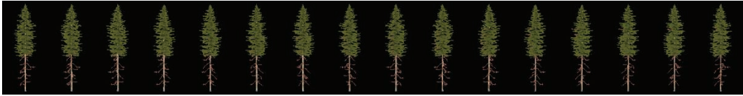
Figure 4.4. A series of 16 orthographic views are rendered to the billboard texture. The closest two views are interpolated between based on camera position.
