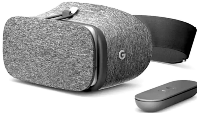
Figure 5.12: Photo credit: Google. One of the attempts that didn't go well with consumers was the Google Daydream headset, which let you drop your mobile phone into this device to do VR. But it wasn't very full-featured; it couldn't do 6DOF, for instance, and only ever had very limited content developed for it.
