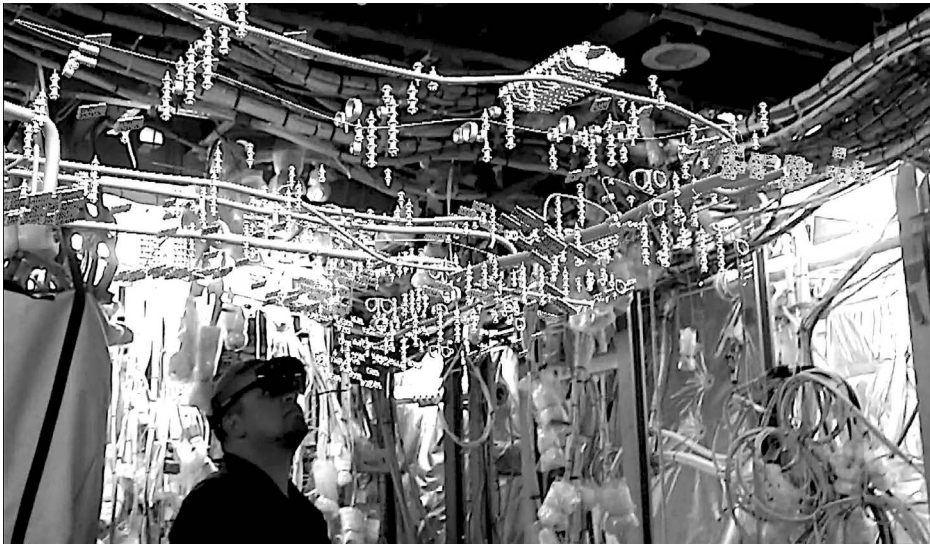
Figure 6.5: Photo Credit: Boeing. Using HoloLens to view a wiring application displaying digital engineering drawings inside a Boeing airplane.
