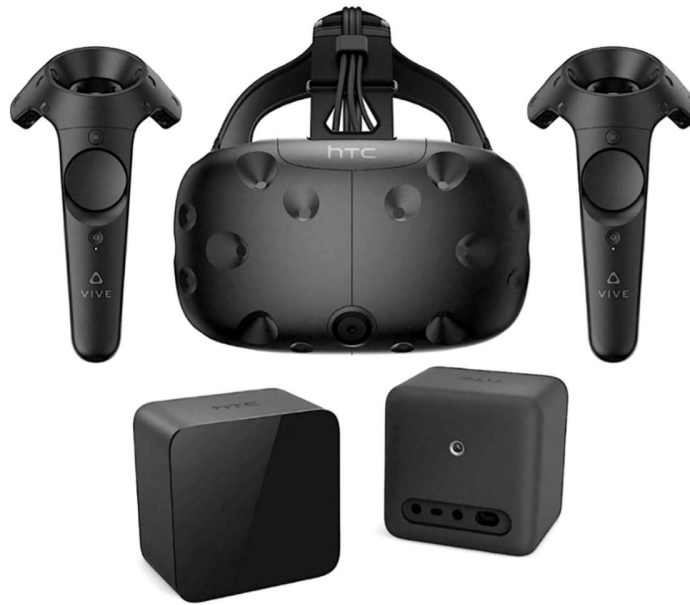
Figure 5.9: Photo credit: HTC. The HTC VIVE and its Lighthouses.
