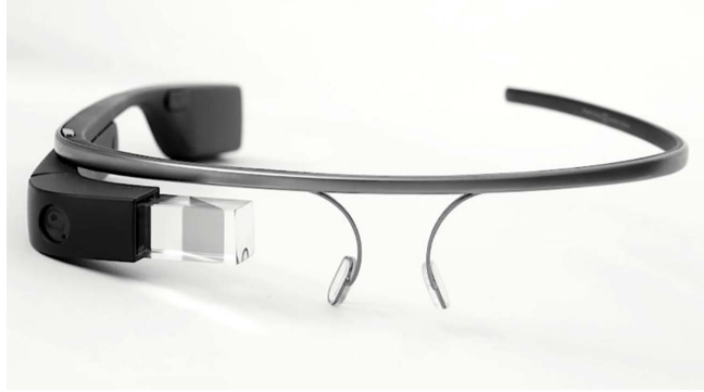
Figure 5.2: Photo credit: Google. Here is a closer look at the original Google Glass, which had a small transparent screen, along with a camera, microphone, speaker, and battery.
