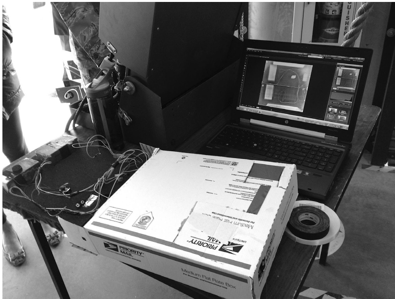
Figure 10.5: A defused bomb for training purposes at Nellis Air Force Base with an X-ray of the scan. (photo credit: Robert Scoble)
