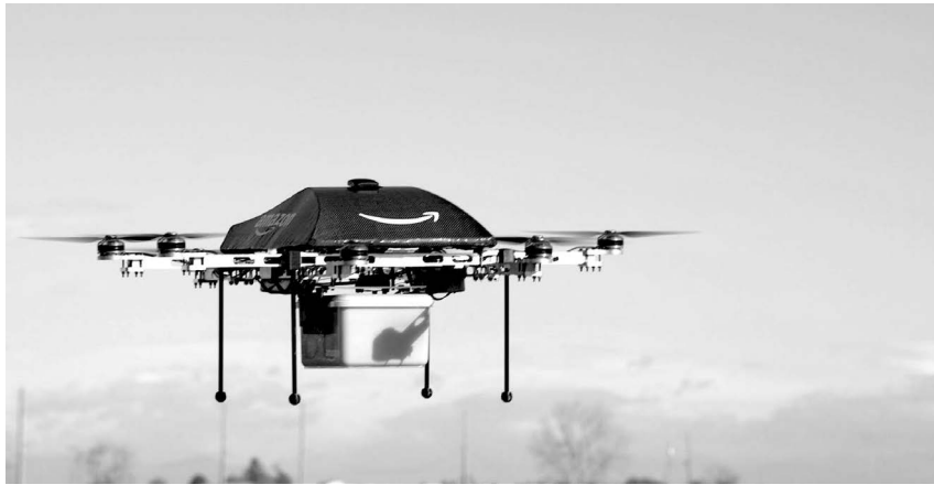
Figure 7.10: Photo credit: Amazon. An example from Amazon Prime Air: a future delivery system designed to get packages to customers in 30 minutes or less using unmanned aerial vehicles, also called drones.
