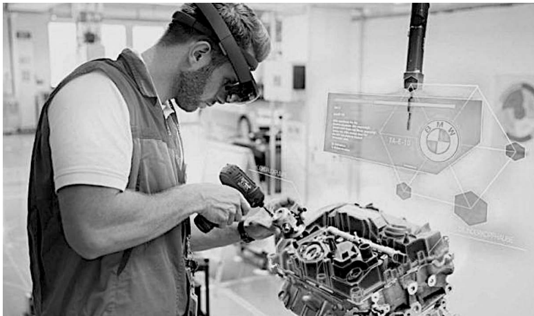
Figure 6.3: Photo credit: BMW. Using a HoloLens to put together a BMW car engine.
