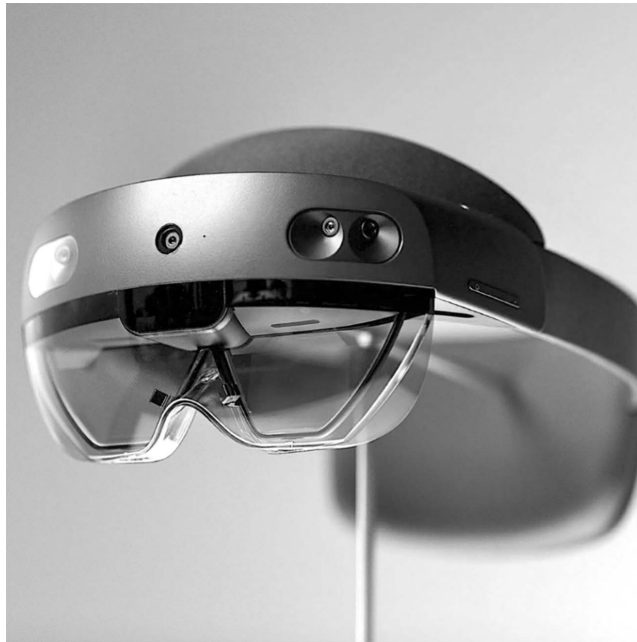
Figure 5.21: Photo credit: Microsoft. HoloLens 2 brings a much more comfortable headset with way better gesture recognition, along with a flip-up screen so workers don't need to remove it as often.
