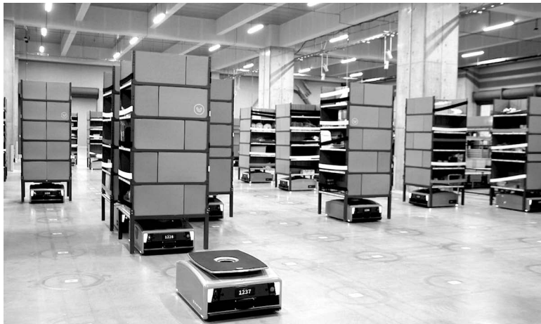
Figure 7.5: Photo credit: GreyOrange. GreyOrange Butler robots working inside a warehouse.
