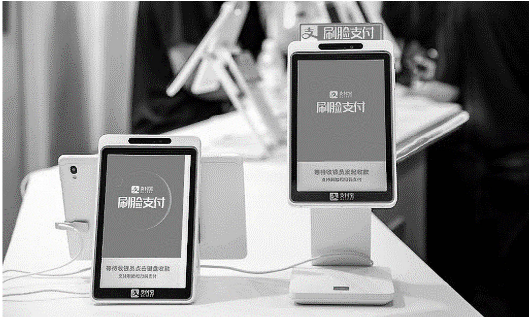
Figure 9.9: Photo credit: Alipay. Pictured here are two Dragonfly facial recognition systems, which are currently actively used in China to make mobile payments.
