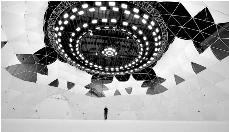
Figure 5.26: Photo credit: Intel Studios. This volumetric capture dome had 100 4K cameras around the dome, all pointed inside. When joined together, the cameras make a 3D image set that you can walk around, or through.
