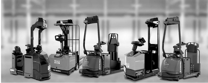
Figure 7.4: Photo credit: Seegrid. Examples of Seegrid's VGVs that replace human-manned forklifts.
