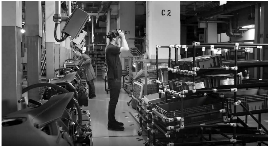
Figure 10.6: A worker uses VR to both build and train on a new manufacturing line (photo credit: BMW)
