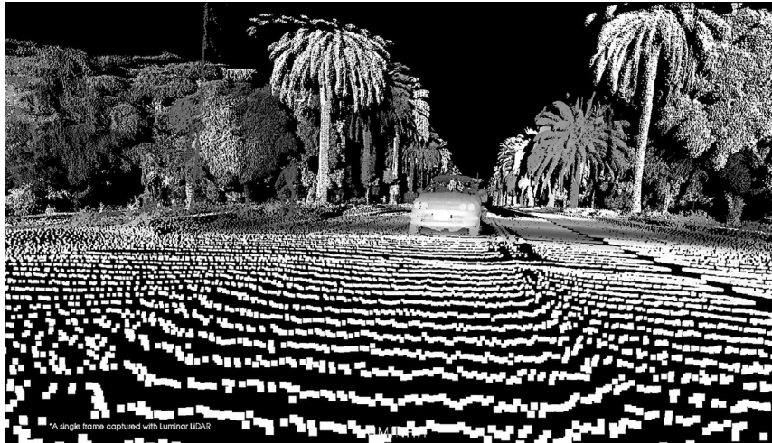
Figure 2.7: Here, a street is mapped out in 3D by Luminar Technologies' solid-state LIDAR.
