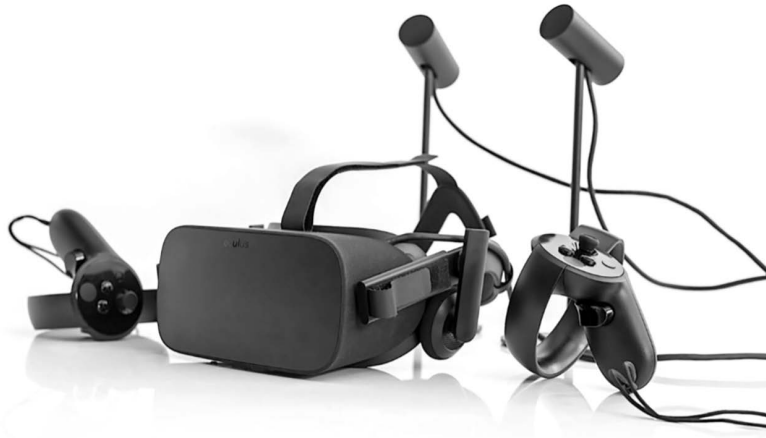
Figure 5.8: Photo credit: Meta. The original Oculus Rift VR system, with its two sensors and controllers.
