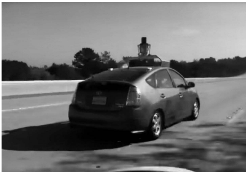
Figure 4.1: Photo credit: Robert Scoble. Early image of a Google self-driving car (now branded as Waymo) on Freeway 280 near Palo Alto with an early-model Velodyne LIDAR system on top, spinning furiously away back in December of 2009.
